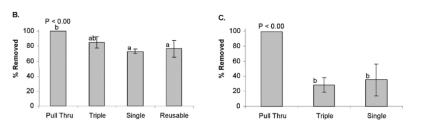
Figure 3. Percent of soil removed (Mean  $\pm$  SD) from the lumen after passage of the lumen-cleaning device.: A. 2.8 mm (new) lumen, B. 2.8 mm (old) lumen, C. 5.0 mm (old) lumen.
